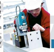
As the cutter bores through the metal, the sprung pilot rod gives way until cutting is completed when the action of the spring immediately ejects the slug.
